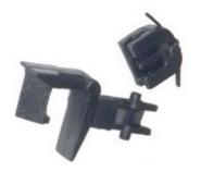
N scale modellers have had a very different type of tension lock coupling, the Rapido coupler. It works like the Tri-ang coupler but with a sideways hook that is pivoted. It is significantly larger, relative to the scale, than modern OO ones and despite its effectiveness is often replaced by modellers looking for more realism in their rolling stock.
