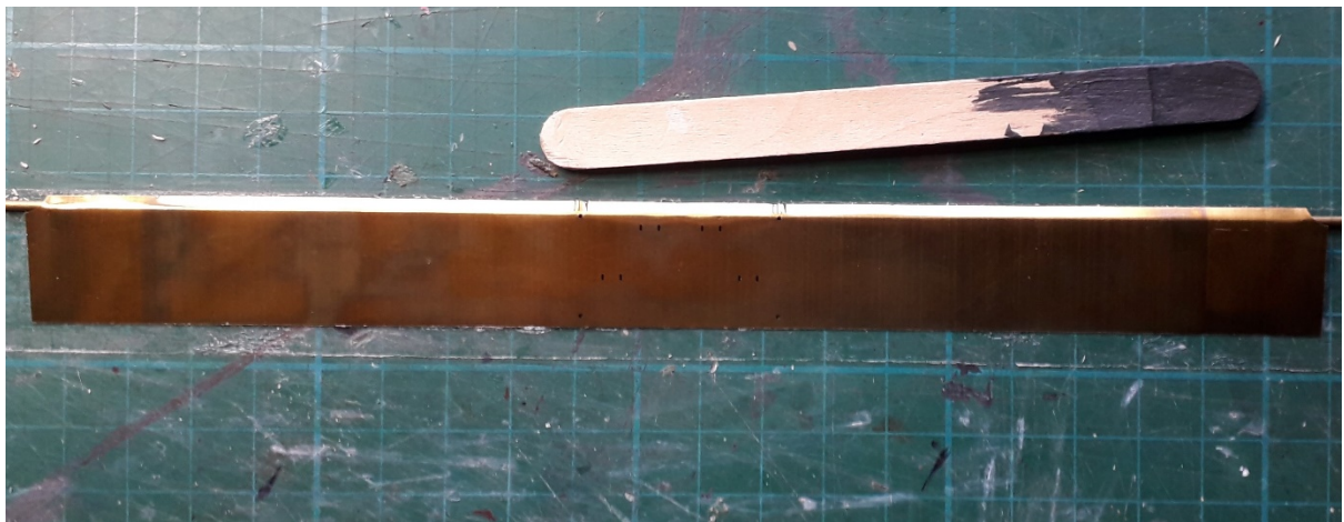
Picture 4. The top edge is rolled over the tube using a wooden lolly stick as a caul.
